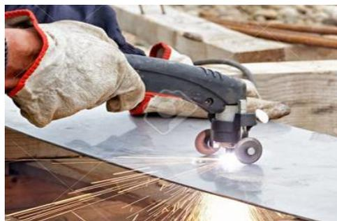
Assist yourself by using a straight bar or angle iron to rest the torch towards when doing straight cuts. Instead of drag-shield, you can also use a roller guide to maintain a consistent standoff. It makes cutting straight line with a handheld plasma cutter easy.
