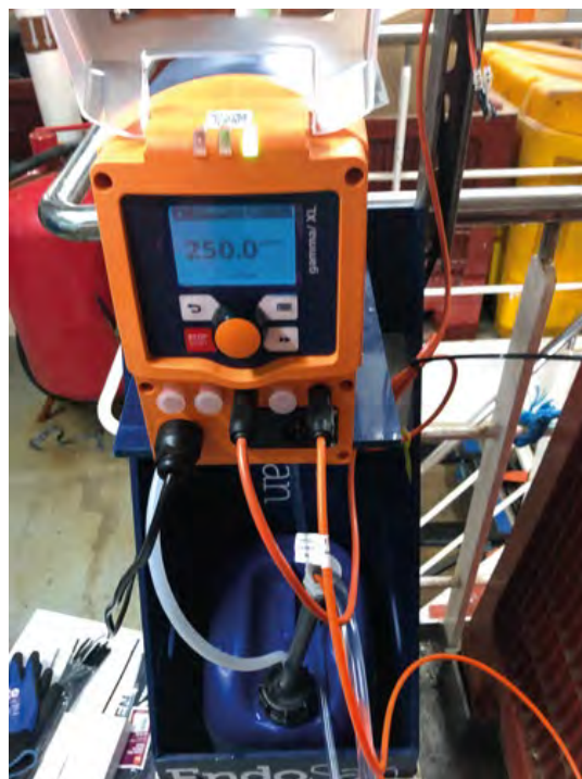
Top down view of the dosing system in operation at 250ppm dose rate
