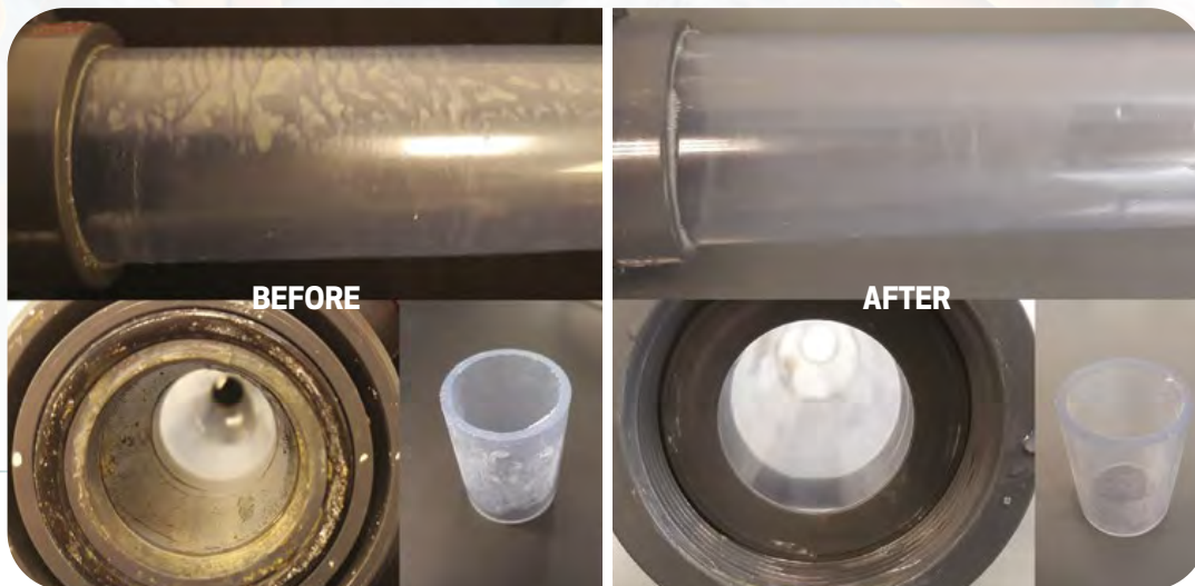
Figure 1 – Visual appearance from the outside of the tube (top) inside the water system (bottom left) and on the inserts (bottom right) before (left) and after (right) the continuous addition of EndoSan to the water.
