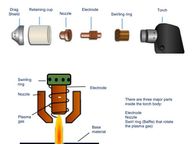
These items are consumed over time during use and must be replaced. The electrode is connected to the negative side of a DC plasma power source. The nozzle is connected to the positive side for arc start, but is electrically isolated while cutting as the work piece is the positive side connected to the power source through the return cable.
