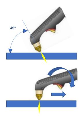
Pierce cuts are a little more difficult. The torch will need to be angled slightly over the starting point. This will prevent the molten metal from the beginning of the cut from being blown back into the tip and electrode.
