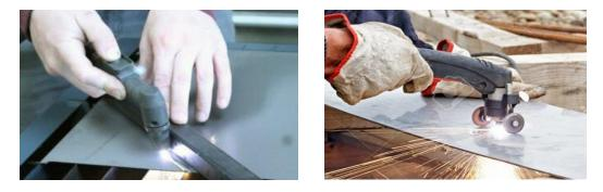
Assist yourself by using a straight bar or angle iron to rest the torch towards when doing straight cuts. Instead of drag-shield, you can also use a roller guide to maintain a consistent standoff. It makes cutting straight line with a handheld plasma cutter easy.
