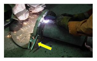
Try to place the return clamp as close to the cut line as possible. If possible, place the clamp on the workpiece itself. Inspect the cables for loose connections, worn spots, or anything else that might resist the electrical flow. Only secure the return clamp to clean metal for getting the best cutting performance. Grind off the paint or rust before clamping as these may inhibit the flow of electricity.
