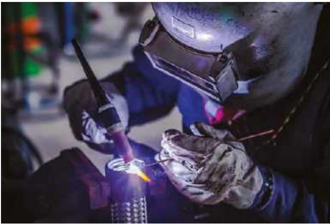
TIG welding equipment
