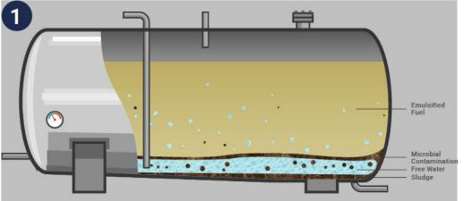
Firstly, identify the current state of the fuel and storage tank. While performing a visual inspection, if the fuel is hazy to a point where you cannot distinguish the inside of the tank, here are some options for you:
