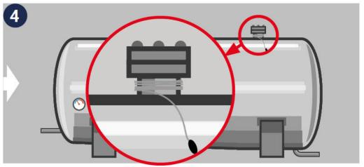
Ensure that sufficient length of cord is left outside the tank so that it can be attached, e.g. by making a loop around the filler pipe, or other suitable secure attachment
