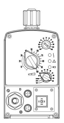
To prime the pump, set the stroke length to 100% and the multifunctional switch to 100% manual.
